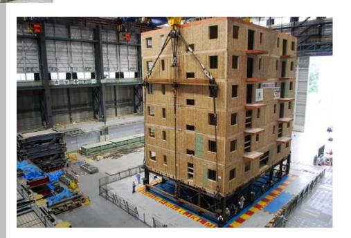
In July 2009, Simpson Strong-Tie in collaboration with researchers from Colorado State University conducted a 7.5 magnitude test on a seven-story wood-framed condominium tower – the largest seismic test ever. Image: Simpson Strong-Tie.
